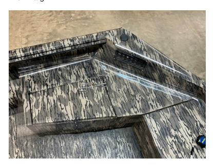
4. With the material roughly laid out, tape one side, pull it snug on the opposite side to remove any bubbles or wrinkles, then secure with tape and repeat.
