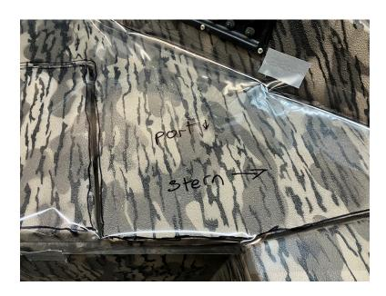
8. One last thing before you remove the tape and prepare for sending, mark every hole for latches or light outlets.
