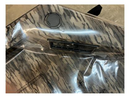
9. If you must tape two sheets together, you should apply the tape every about every foot, and mark it as shown. Using a straight-edge mark on either side of it in at least two locations, as well as some diagonal tick marks along the seam.
