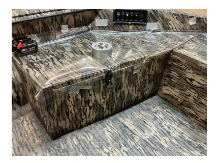
5. If wrapping the excess up a wall, you might want to use a weight close to the wall to keep a ramp from forming. Also in corners, a relief cut may be necessary for the material to lay flat.
